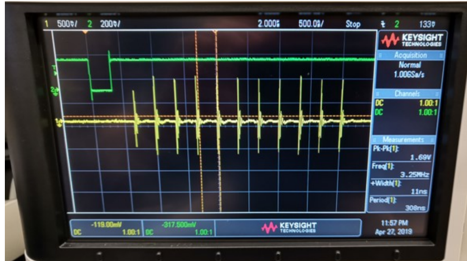
Figure 4.16: Power trace of AES-128 encryption implemented on Kintex-7.
