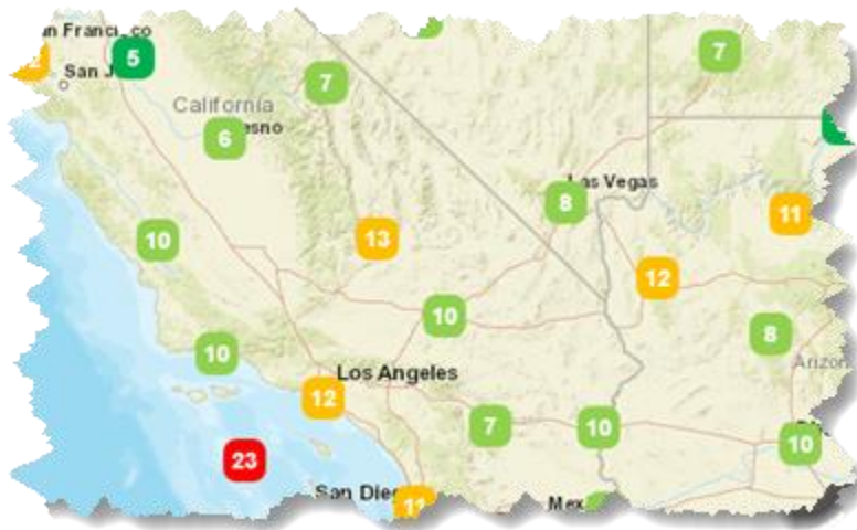
Figure 38. Prevailing surface wind markers (in knots) as displayed on the map for southern California depicting NBM forecasts at some departure time as set on the departure advisor.
