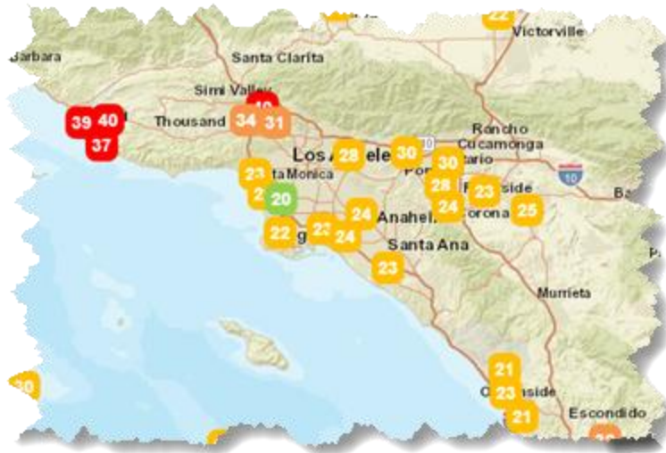
Figure 40. Surface wind gust markers (in knots) as displayed on the map for the Los Angeles area depicting NBM forecasts at some departure time as set on the departure advisor.
