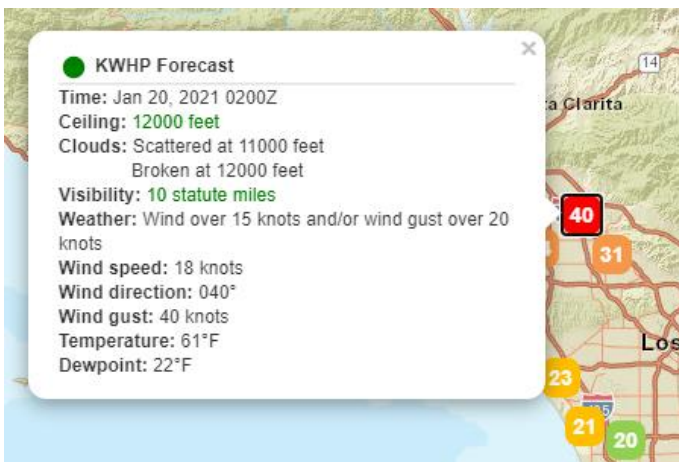
Figure 35. Each station marker provides essential weather information (observed or forecast) to include the valid time of the observation or forecast, ceiling height, cloud coverage, surface visibility, predominant weather, prevailing wind speed, prevailing wind direction, wind gust, surface temperature and surface dewpoint temperature.
