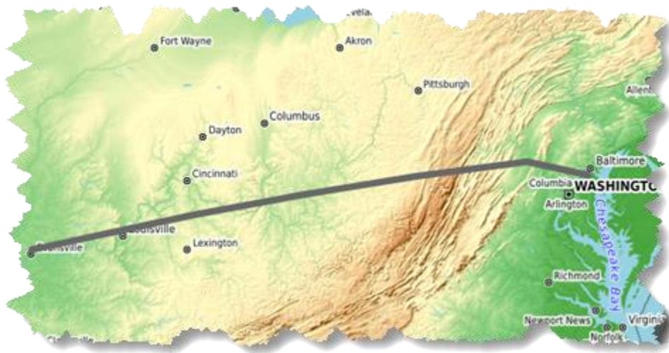
Figure 31. Topographic base map showing a great circle route (gray) plotted from Baltimore/Washington International Airport (KBWI) to Evansville Regional Airport (KEVV) via the Martinsburg, W.Va. NAVAID waypoint.
