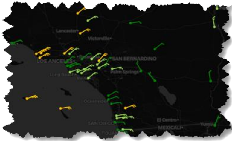
Figure 39. Prevailing surface wind barbs (wind speed and direction) as displayed on the map for southern California depicting NBM forecasts at some departure time as set on the departure advisor.
