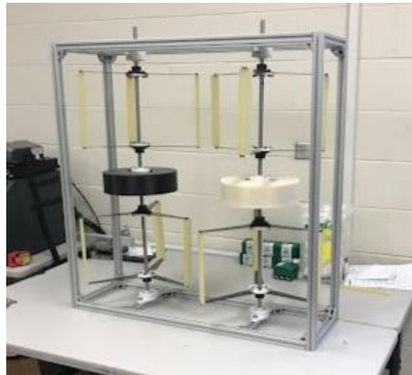
Figure 4. Photograph of the assembled DD-VADHT scaled prototype.
